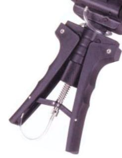
The 411 Hand Pump is ideal for testing, commissioning and maintaining pressure gauges, pressure sensors and pressure switches. Thanks to its ergonomically designed handle, this unit sits easily and comfortably in the hand. The rotating head permits optimum readout from pressure gauges and the fine regulation feature enables precise pressure and/or vacuum adjustments to be made.
